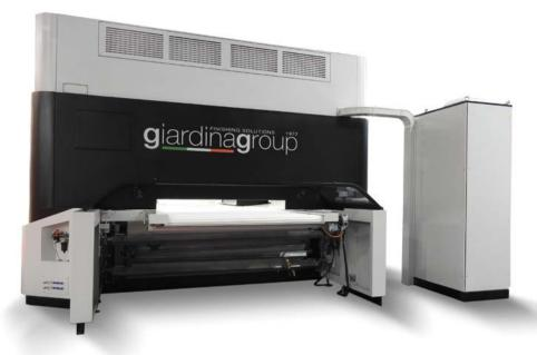
processed by the management software, is transmitted to the guns as ON or OFF signals. The dimensional reading device for the parts to be painted scans every 5mm to optimise the painting phase and reduce consumption. Lastly, Dualtech Forma is equipped with an environment air supply and filtration unit, and can be fitted with an air heating and air conditioning system on request.
