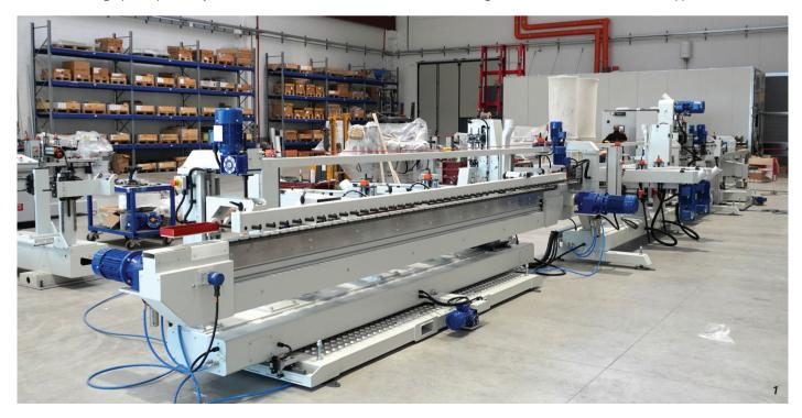
sanding, a CTL100x unit for lateral transversal sanding, a CTS200 unit for upper longitudinal sanding, two AT100 units for sanding straight or shaped parts, and an SB100 unit, a brush honing unit or an abrasive wheel honing unit suitable for super-finishing, satin finishing and brushing of sanded surfaces. If necessary, a seventh unit can be added.
