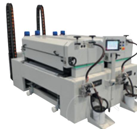
Two heads roller coater with one direct application unit
