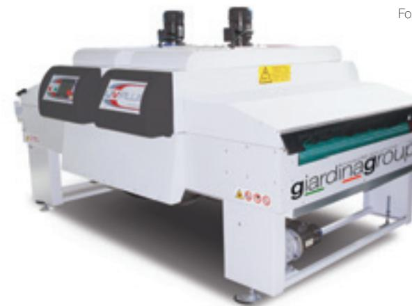
Gst ultraviolet curing tunnel Albatros with cold reflection
