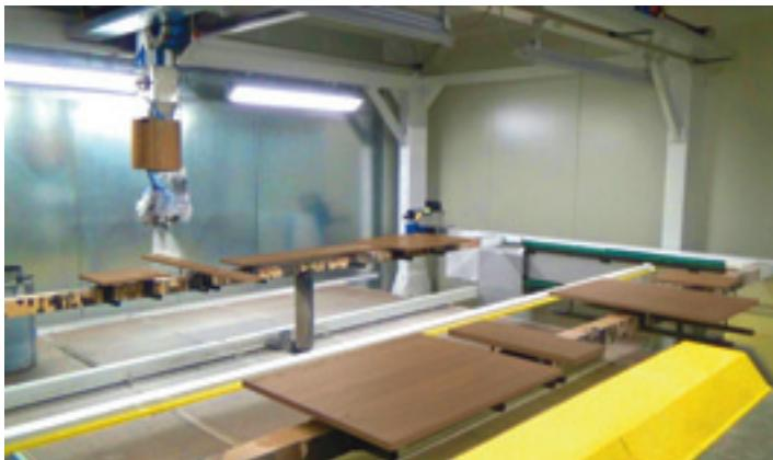
Spraying robot for panels
