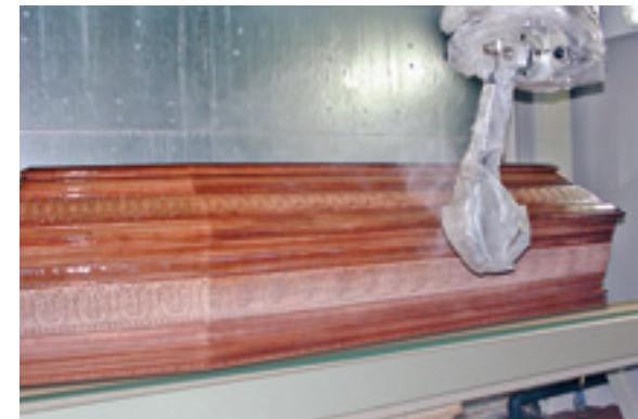
Finishing robot for assembled pieces
