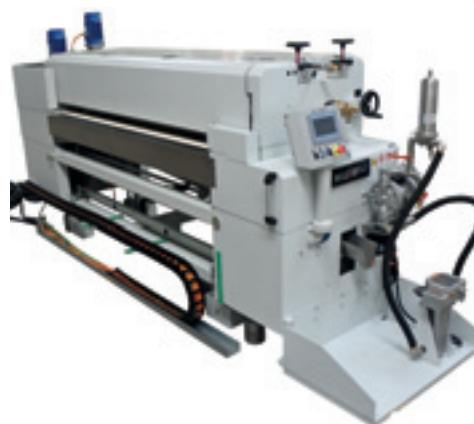
Precision roller coater with reverse dosing roller type G02-05-2200
