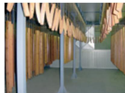
Assembled suspended frame coating
