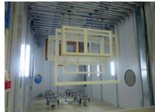
Finishing installation with overhead conveyor
