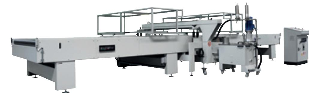
Curtain coater with double bed and two coating heads on removable trolleys
