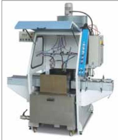
tem of air extraction and filtering. The transport system is made by two guided feed belts with speed adjustable by inverter. The machine can be equipped with 3 or 4 guns and the spraying operation is controlled by an efficient electronic system. ■
